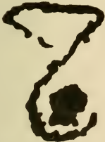
Between Worn Wheel and Worn Rail
